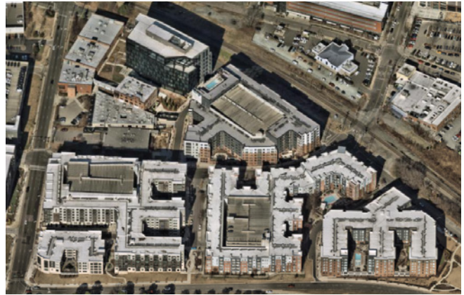
Parking garages near downtown Durham sited at the center of blocks and wrapped with buildings.
