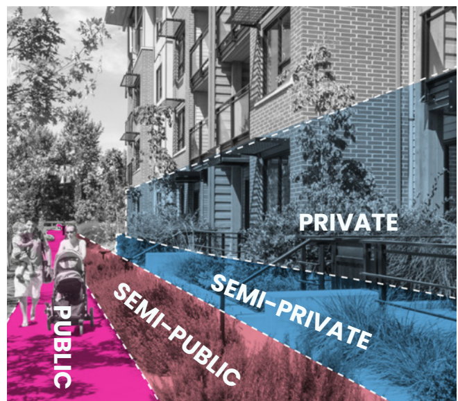
A transition from the public to private realm within the frontage zone.
